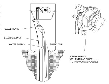
CAUTION: Installation must not cause any strain on heater wiring connections. Do not cross the cable over itself along the water supply line. Avoid heater damage caused by hot spots due to its leads lying close to each other. Also, do not wrap additional insulation around heater.
