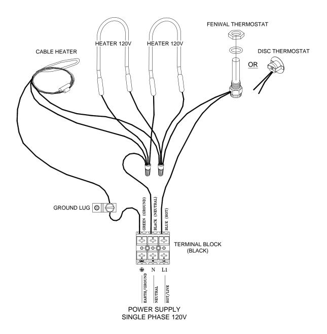
NOTE: National/Local electrical codes may require livestock waterers installed in feedlots in open feeding area to be grounded by a separate stranded copper grounding conductor or at least no.6 AWG terminating at a point where the branch circuit receives its supply. Check with local inspecting authorities.
