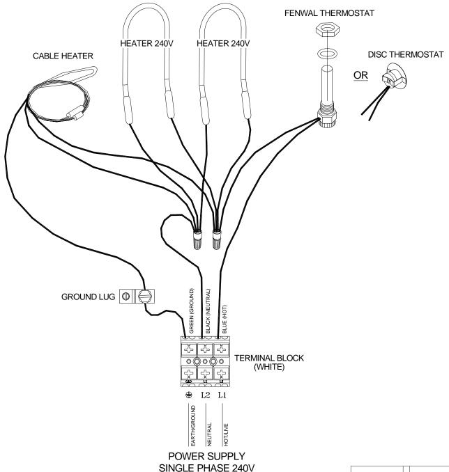
**L. Terminal Block** – The terminal block is provided for easy and quick connection to the power source. The push buttons provide quick connection with a screwdriver or by hand. If you are using solid wire then you will be able to just push the wire into the slot. Stranded wire will require you to press the button down.
