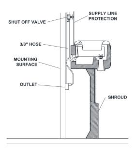
D. Water Supply Through Wall - Through wall supply lines should be sized to account for pressure drop, relating to distance, and located to prevent tampering by livestock. A one-inch supply pipe is recommended. A shut-off valve should be located at the fountain to allow for servicing. If your facility is cold in the winter, additional cold climate protection will be required.
