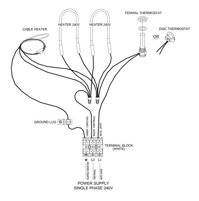
J. **Terminal Block** – The terminal block is provided for easy and quick connection to the power source. The push buttons provide quick connection with a screwdriver or by hand. If you are using solid wire then you will be able to just push the wire into the slot. Stranded wire will require you to press the button down.
