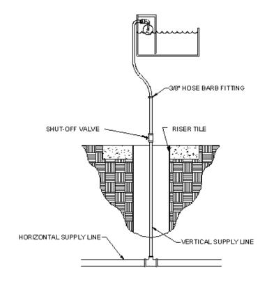
the fountain to allow for servicing. If your facility is cold in the winter, a using a Ritchie Thermal Tube as your riser will provide optimum protection to the vertical supply line against frost and freezing.
